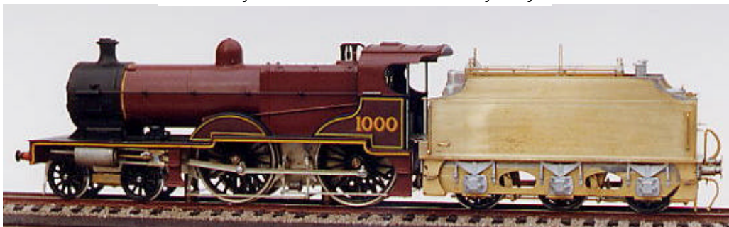
LCP9 LMS Compound 4-4-0, with Hornby body and TK7 tender kit, a Fowler 3500 gallon flush riveted tender.
