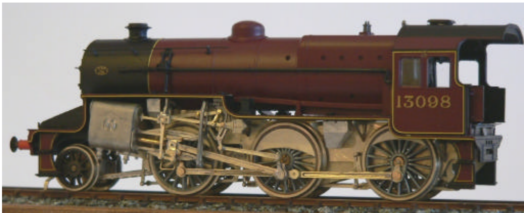
LCP14 , LMS Crab with Walschaerts valve gear. Seen here under a Bachmann body.
