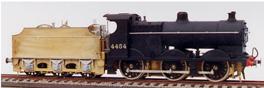
LCP6 Fowler 4F with TK7 tender kit. TK7 is a Fowler 3500 gallon flush riveted tender. This picture shows the tender built without coal rails and with an Airfix/Hornby body moulding
