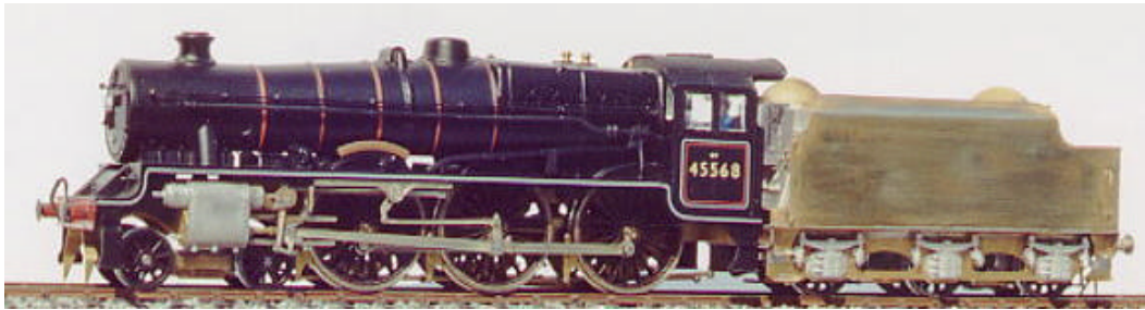
LCP1 (with a TK2) for Royal Scot, Jubilee or Patriot. Seen here with a Mainline Jubilee body. TK2 is a Stanier 4000 gallon welded tender
