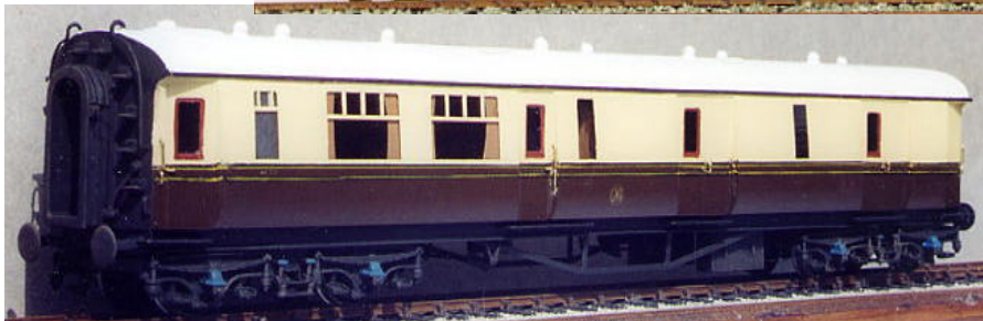
W73 60' Corridor Brake Third Right Hand Dia D120 1935
